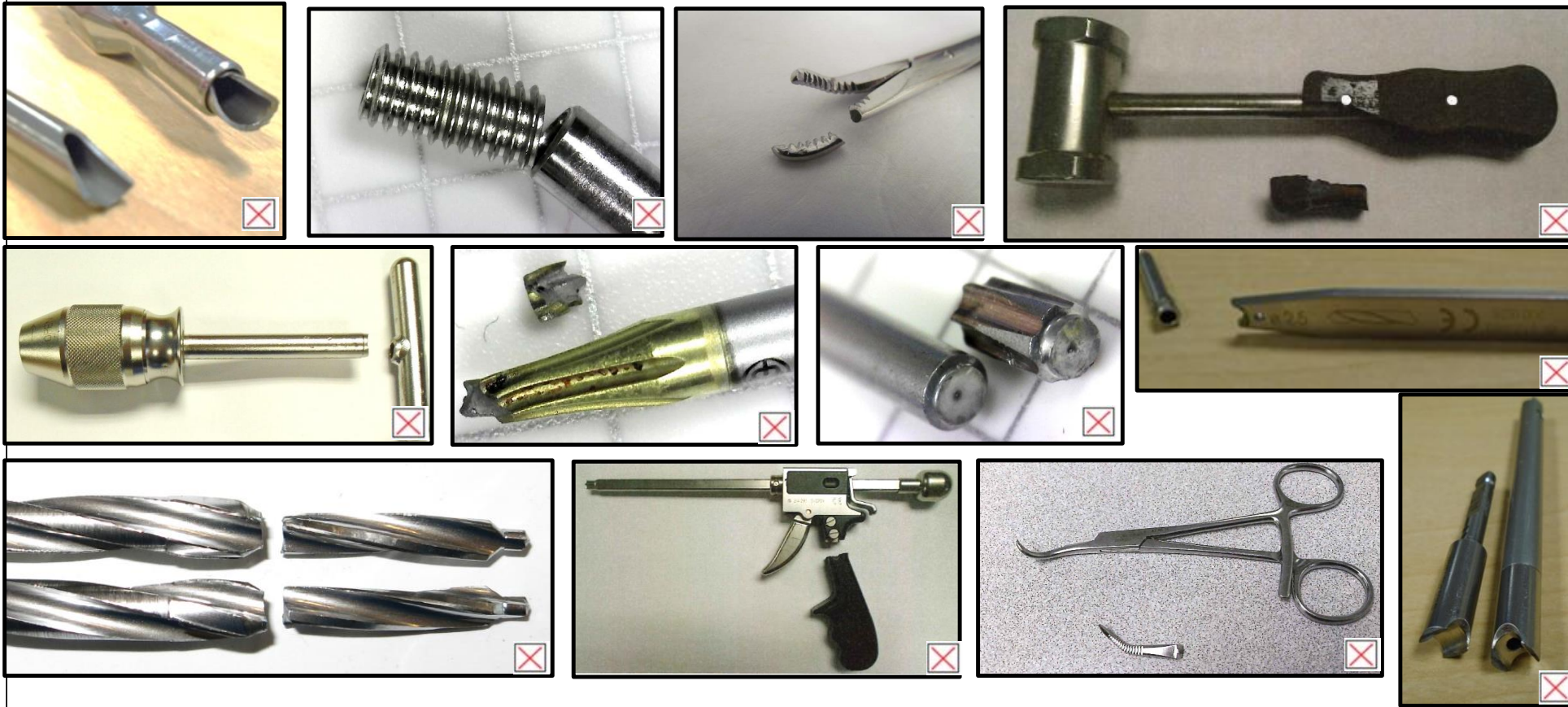
EOLi: Broken at welded joints, driver/tip breakage, broken at assembly joints (e.g., Plastic handles)
